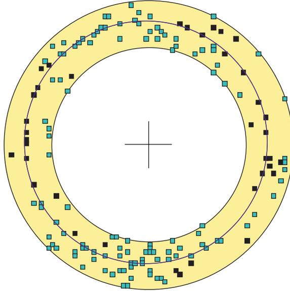
Figure 4: Search area for the target track indicated in Fig. 3 under the correct—pion, in this case—hypothesis. Hits filled in blue have substantial flux ( $\beta_i \geq 10$ ) from background tracks. Circles corresponding to the target Čerenkov ring fitted by a full, non-linear fitting algorithm and the linearized approximation are shown. The two fits are identical within estimated errors. Width of cross at center indicates  $\pm 10$  mrad.
