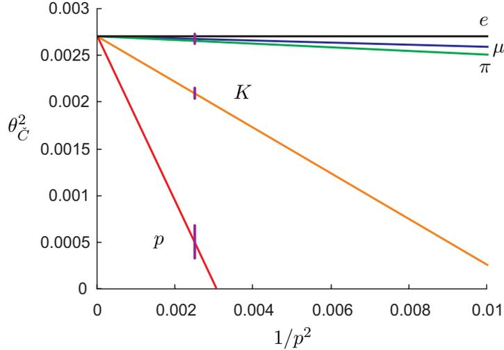
Figure 10:  $r2p2$  plot showing  $2\text{-}\sigma$  widths of bands for a 20 GeV/c track (purple vertical lines). The  $e, \mu, \pi$  bands are merged at this momentum.
