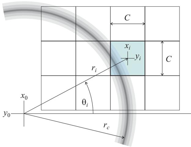
Figure 2: Schematic drawing of Čerenkov photon intensity distribution overlying a set of detector cells.
