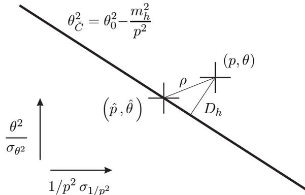
Figure 9: Schematic representation of a Čerenkov band for hypothesis  $h$  on the  $r2p2$  plot indicating a point at the “true” values of momentum and Čerenkov angle and a point corresponding to the measured values,  $(p, \theta)$ . The quantities  $\rho$  and  $D_h$  are defined in the text.
