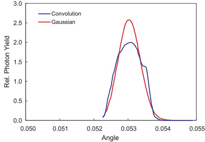
Figure 1: Blue curve: a calculation of the expected Čerenkov-angle distribution of photons detected with the HERA-B *RICH*. The “shoulder” on the right side is due to the absorption properties of the lenses used for collecting and imaging light onto photomultipliers. Red curve: a Gaussian distribution with the same mean and standard-deviation ( $\sigma_d = 0.34$  mrad).
