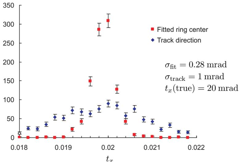
Figure 7: Histogram of horizontal track direction (ring center)  $t_x$  from likelihood fits using a soft momentum constraint for 20 GeV/c particles—the true particles are pions. Fits were performed with backgrounds as depicted in Fig. 3. Notice that the fitted resolution in one-dimension of track direction is approximately  $\sqrt{2}$  times the resolution in fitted radius (see Fig. 6), as expected for rings fully contained within the *RICH* acceptance.
