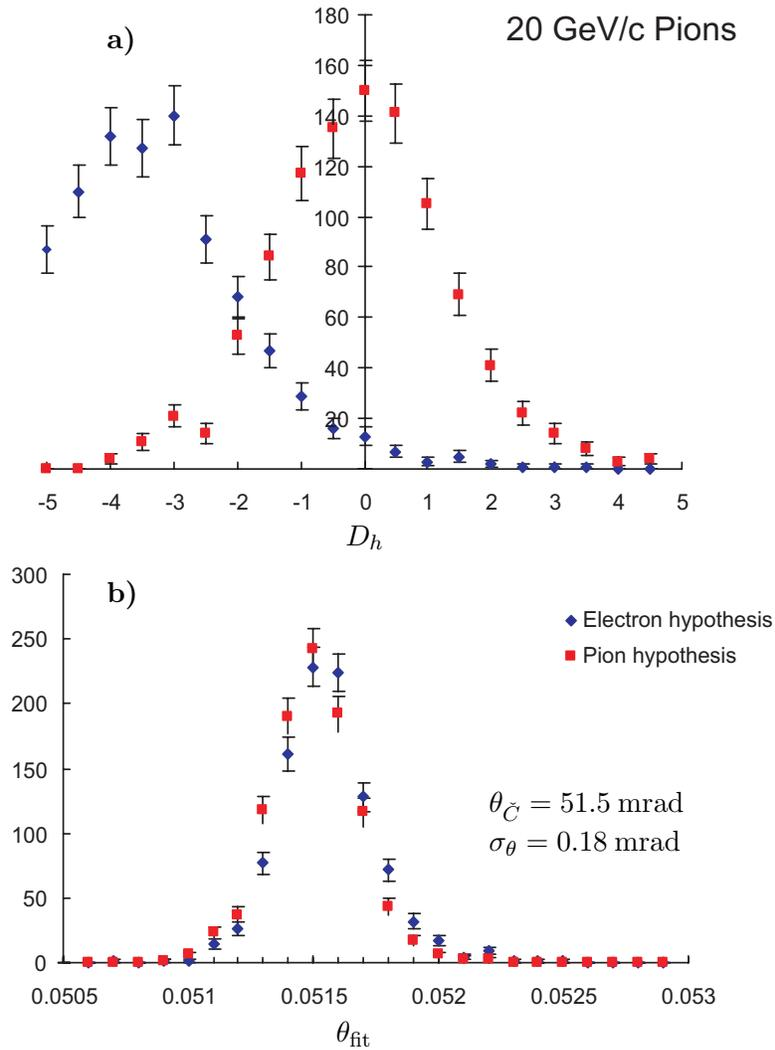
Figure 6: Results of likelihood fits using a soft momentum constraint for 20 GeV/c particles—the true particles are pions. Histogram a): number versus the  $r2p2$  distance  $D_h$  for pion and electron hypotheses. Histogram b): number versus fitted Čerenkov radius for pion and electron hypotheses. Fits were performed with backgrounds as depicted in Fig. 3.
