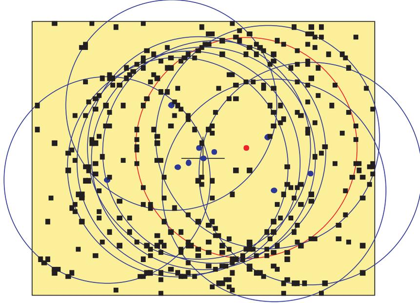
Figure 3: Photon detector image-plane view of Čerenkov photon hits from a typical monte carlo event used in the studies discussed here. Circles corresponding to expected Čerenkov rings are shown. The red ring corresponds to the target track being fitted. Width of cross at center indicates  $\pm 10$  mrad.
