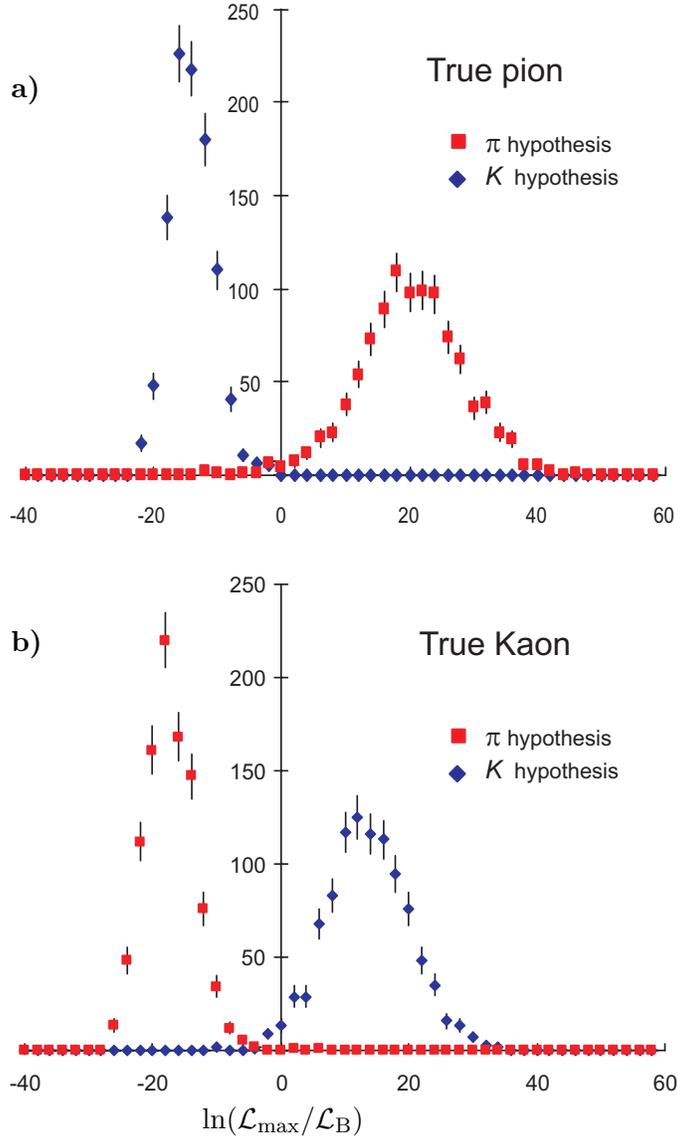
Figure 8: Results of likelihood fits using a soft momentum constraint for 20 GeV/c particles. Histogram a): number versus  $\ln(\mathcal{L}_{\max}/\mathcal{L}_B)$  for pion and kaon hypotheses when the true particles are pions. Histogram b): number versus  $\ln(\mathcal{L}_{\max}/\mathcal{L}_B)$  for pion and kaon hypotheses when the true particles are kaons. Fits were performed with backgrounds as depicted in Fig. 3.
