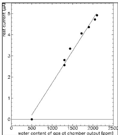
Fig. 5. Measurement of dark currents versus the water concentration. An almost linear dependency of the ohmic dark current with the water concentration is observed. The gas used is Ar/CF<sub>4</sub>/CO<sub>2</sub> (65:30:5).
