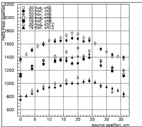
Fig. 6. Peak position of the <sup>55</sup>Fe spectrum along the wire for several irradiated wires after an accumulated charge of 600 mC/cm in chambers operated with Ar/CF<sub>4</sub>/CO<sub>2</sub> (65:30:5) (full symbols), compared with the situation before irradiation (open symbols). The gain drop is between 6-10 % in the center of the irradiation zone due to the swelling of the anode wires.
