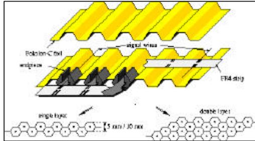
Fig. 1. Illustration of the honeycomb technology. See explanations of the building technique in the text. In the lower part of the figures, the cross section of single and double layers modules are shown.
