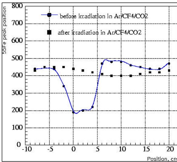
Fig. 4. Position of the  $^{55}Fe$  peak as function of the source position along the wire after severe anode aging produced by irradiation under  $Ar/CF_4/CH_4$  (74:20:6) (full circles and curve) and after recovering from irradiation by operating with  $Ar/CF_4/CO_2$  (65:30:5) (squares).
