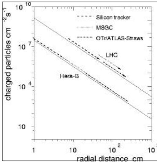
Fig. 2. Comparison of the primary charged particle density as function of the radial distance from the beam for detectors at HERA-B and LHC. It can be seen that, at HERA-B, detectors are closer to the beam, thus receiving the same charged particle flux, as LHC detectors will detect.
