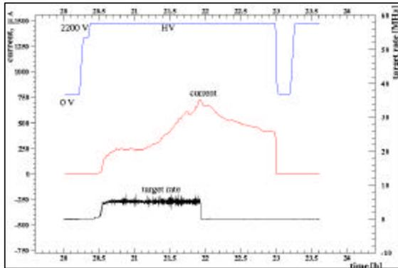
Fig 3. Example of the development of Malter currents in 1997 test chambers installed in HERA-B. The chambers were built with uncoated Pokalon-C foil. The drift gas was  $CF_4/CH_4$  (80:20). The figure shows the time behavior of the high-voltage applied to the anode wire, the anode current measured and the target rate (which is proportional to the radiation load in the chambers).
